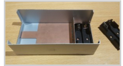
The vertical piece of copper clad separates the battery compartment from the electronics.
