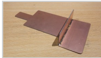
Base plate for the receiver, made of copper clad. I cut away some parts to allow it to place/remove in the case without removing connectors, switches, etc.
