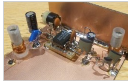
The NE612 mixer with input bandfilter and VFO.
